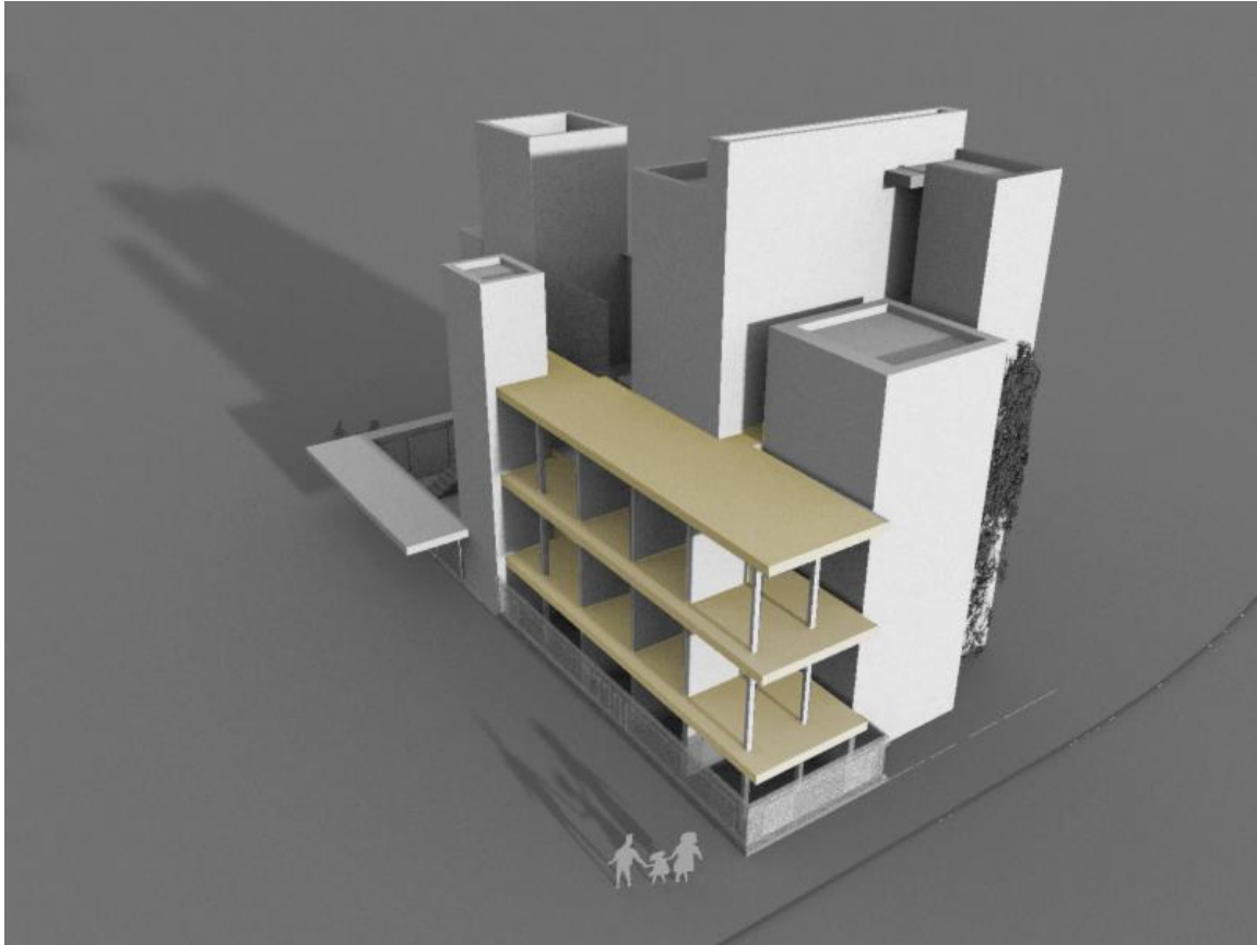
Diagram showing Cross Laminated Timber (CLT) infill for changing room platforms as they relate to plank-formed concrete vertical “stacks”.
